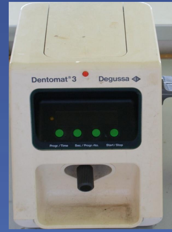
Amalgamator : machine for mixing amalgam: Vibration mixing of alloy and mercury
